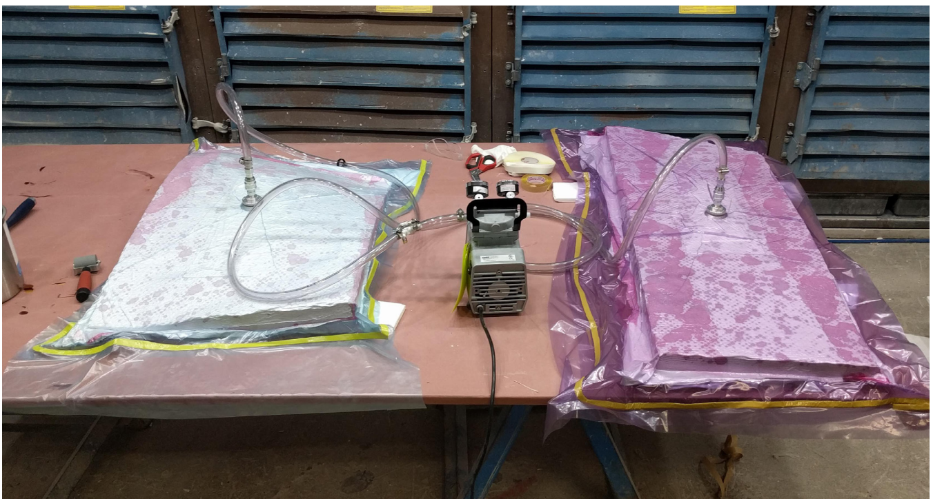
Figure 9. Marble Canopy Fiberglass Lamination and Vacuum Bagging . Photo by Author.
