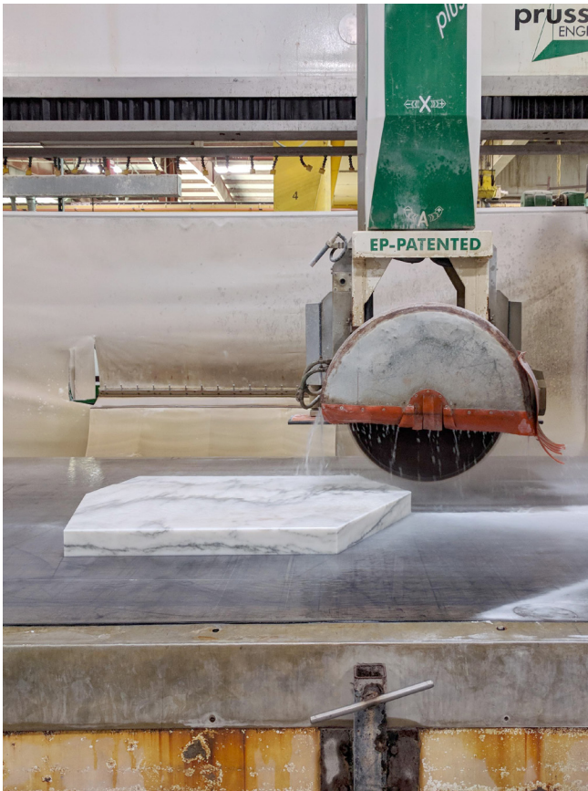
Figure 7. Marble 5-Axis Diamond Blade Machining. Photo by Author.
